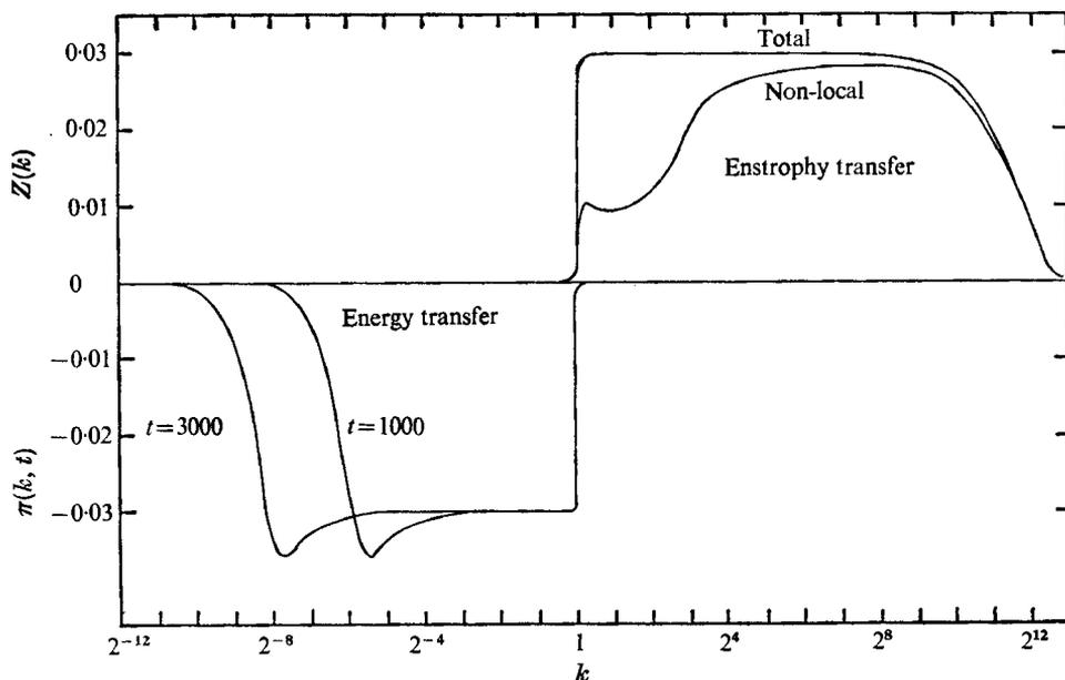
FIGURE 6. Quasi-steady energy transfer rate  $\Pi(k, t)$  and enstrophy transfer rates  $Z(k, t)$  and  $Z_{NL}(k, t)$  for  $t = 1000$  and  $3000$ ; same conditions as in figure 5.
