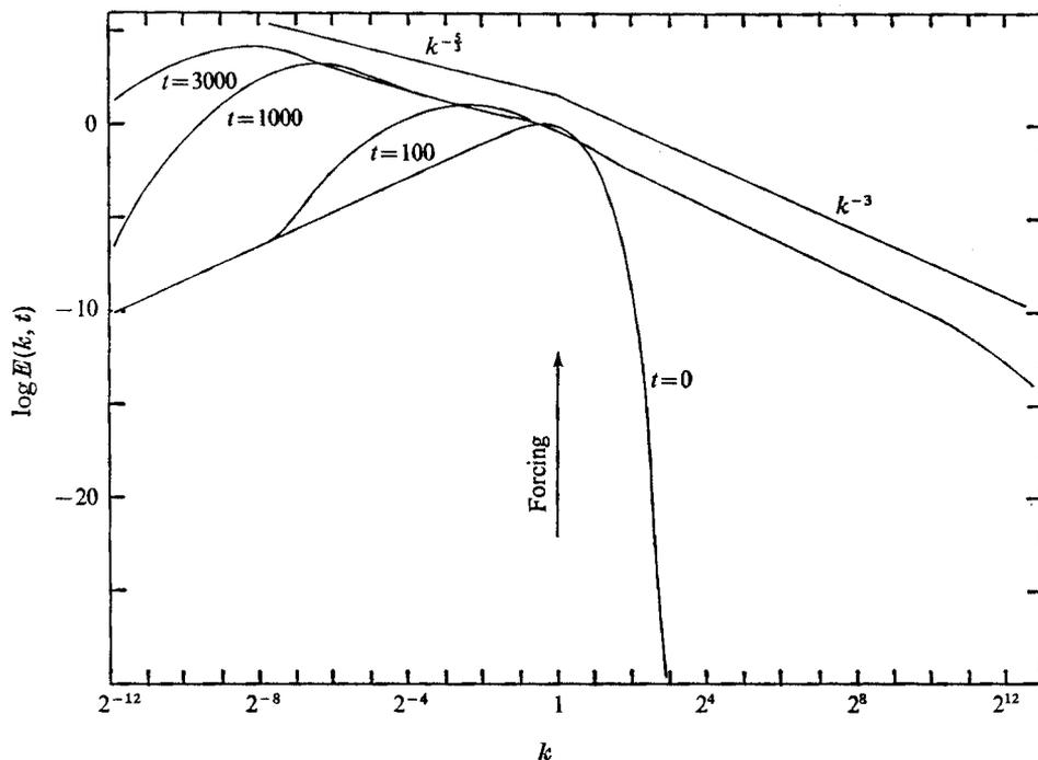
FIGURE 5. Quasi-steady energy spectrum  $E(k, t)$  for  $t = 100, 1000$  and  $3000$  corresponding to an injection spectrum constant in a half-octave band around  $k_I = 1$  with injection rates  $\epsilon = 0.03$  and  $\beta = 0.03$ . Reynolds number  $R = 2.4 \times 10^7$ .
