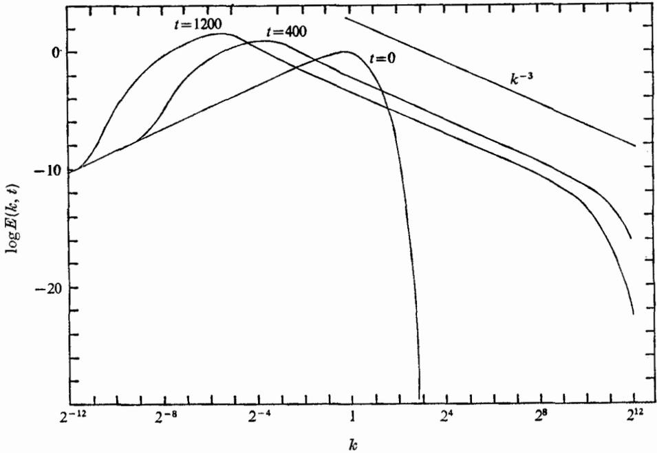
FIGURE 1. Free evolution of the energy spectrum without forcing. Initial spectrum  $E(k, 0) \sim k^3 \exp\{-\frac{3}{2}(k/k_I)^2\}$ . Reynolds number  $R = 2.4 \times 10^7$ .
