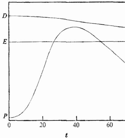
FIGURE 2. Variation of total energy  $E = \langle u^2 \rangle$ , total enstrophy  $D = \langle (\text{curl } \mathbf{u})^2 \rangle$  and total palinstrophy  $P = \langle (\text{curl curl } \mathbf{u})^2 \rangle$  in arbitrary units for two-dimensional turbulence with the same initial conditions as in figure 1.
