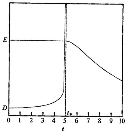
FIGURE 3. Variation of total energy and total enstrophy for three-dimensional turbulence in the limit of infinite Reynolds number. Notice the onset of 'inviscid dissipation' after  $t_*$  (taken from Lesieur 1973).
