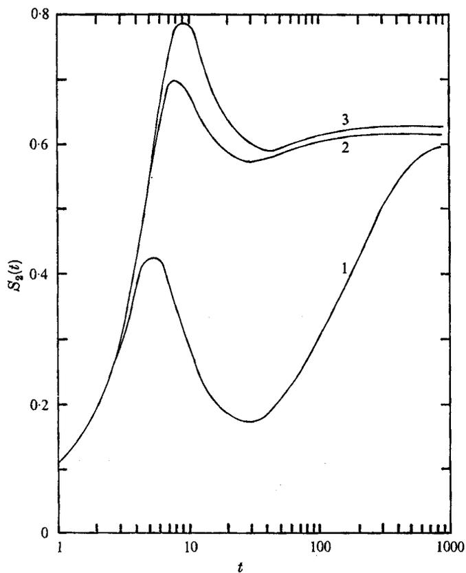
FIGURE 4. Variation of the skewness factor as a function of time for different values of the Reynolds number. Curve 1,  $R = 10^4$ ; curve 2,  $R = 2.6 \times 10^5$ ; curve 3,  $R = 2.4 \times 10^7$ .
